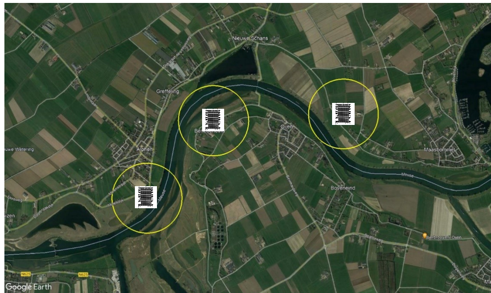
Figure 1 Example of possible interference areas that can have a negative impact on communication on a river, where the maximum emission values according to Table 1 have been adhered to. The circles each have a radius of 500 m, assuming one source of interference (inverter) per location.
