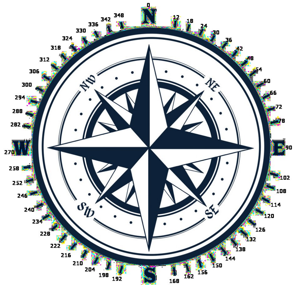
Figure 10. A compass rose where the number of degrees is indicated along the outer edge. The four wind directions are North (0°), East (90°), South (180°) and West (270°).
