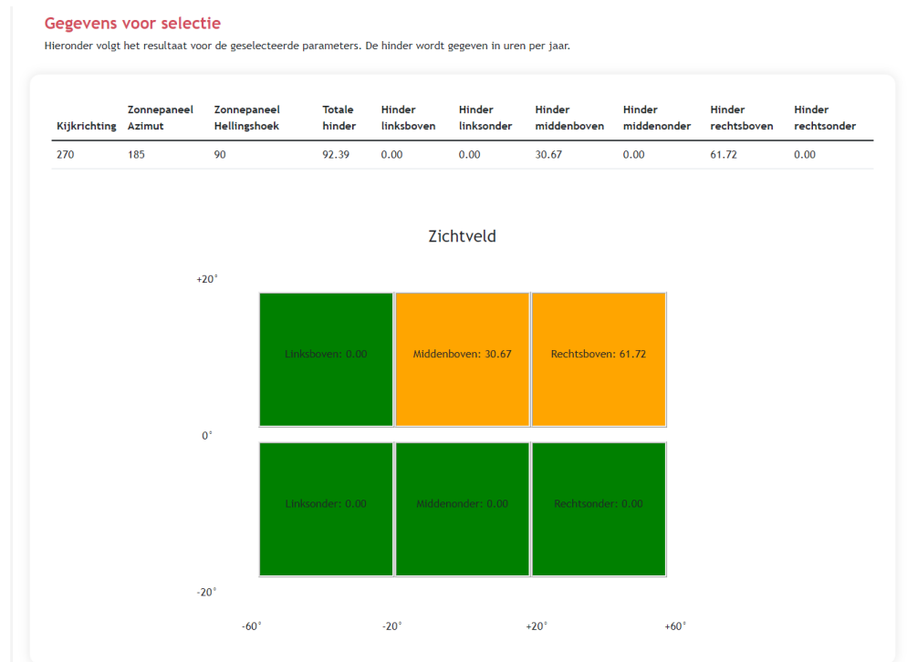
Figure 41 Result of the calculation tool for the proposed solar panels and a western viewing direction. It can be seen that in the right and middle upper part of the field of vision there is a hindrance for this observer.
