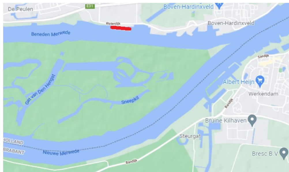
Figure 36 A map with a proposed solar field drawn in red. The solar field is located directly on the quay and is facing the water with the front.
