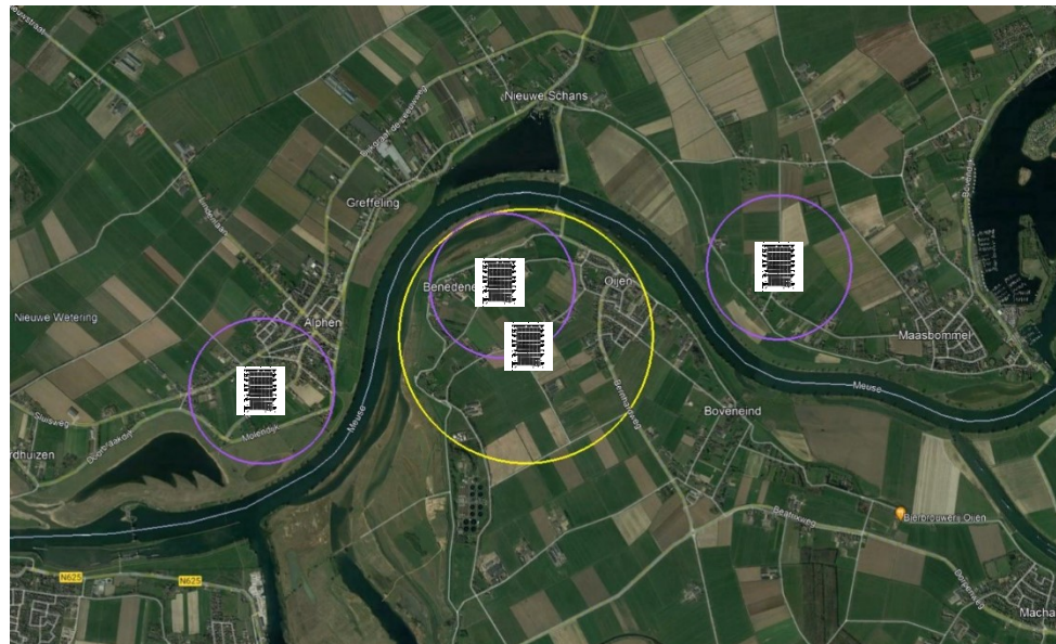
Figure 2 Example where the PV installations have shifted. The purple circles represent locations at a distance of 500 m, the yellow circle the position of an (imaginary) PV installation with more than 1 inverter, and therefore more radiation, where a distance of 880 m must be maintained to stay within the emission standards.
