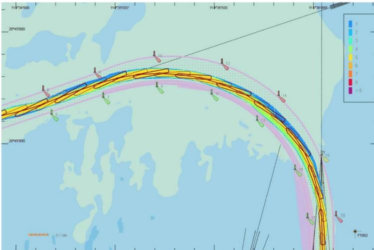
This figure shows the result of a fast time simulation where a cruise vessel has been undertaking several passages leaving a port. One actual track is shown on top of the swept area for all simulations.
