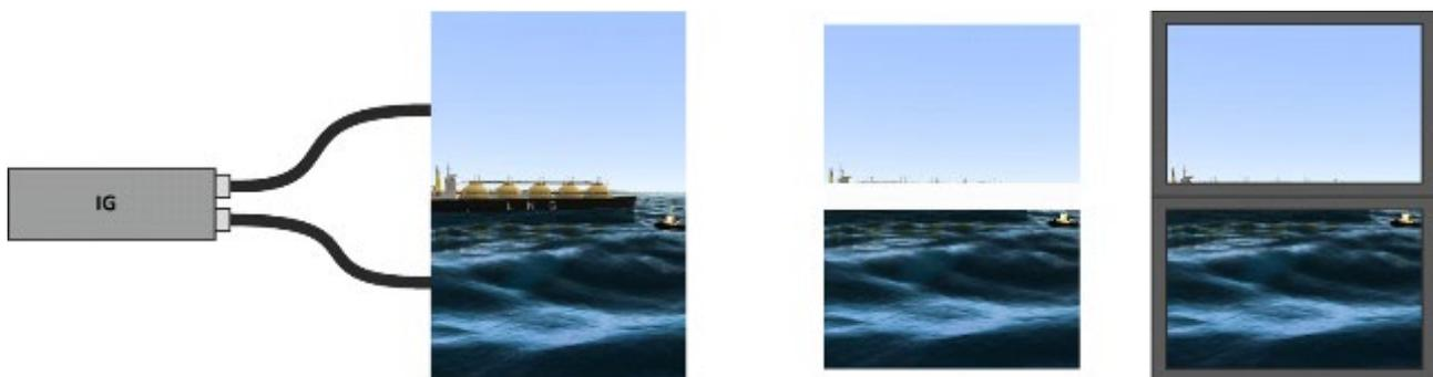
Figure 11 Bezel correction for video walls
