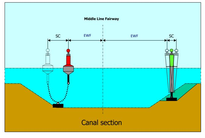
Figure 9 Seekanal Rostock – canal section
