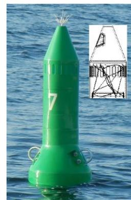
Figure 16 Plastic buoy
