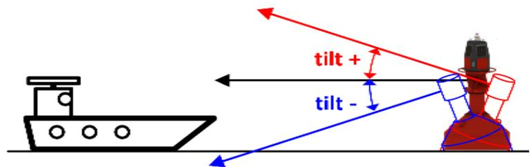
Figure 2 Tilt angle of buoys
