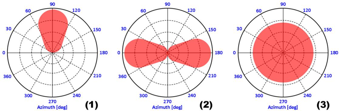
Figure 1 Examples of different horizontal reflection properties
