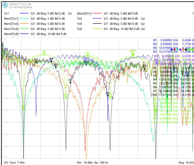
Figure 49 Measurement results, attenuation of plastic samples
