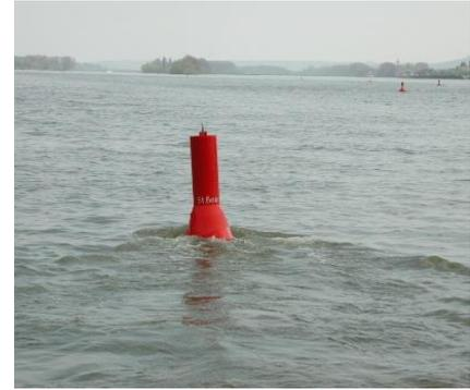
Figure 15 Buoy with fixed orientation to the waterway
