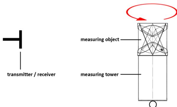
Figure 27 Radar reflector on measuring tower, elevation angle 0°
