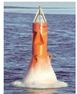
Figure 36 Radar reflector integrated into the buoy body
