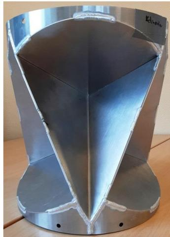
Figure 47 First sample of SR6-330 radar reflector
