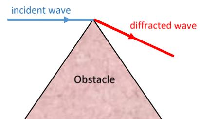
Figure 5 Diffraction
