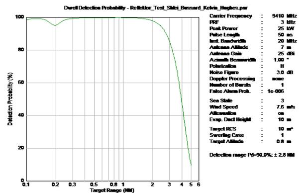
Figure 58 Simulated maximum radar range
