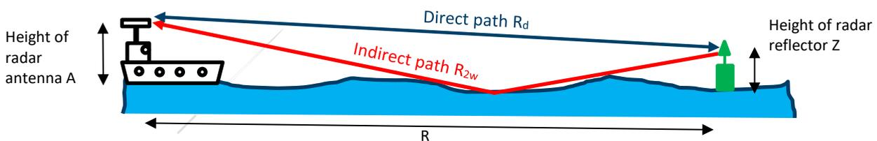
Figure 8 Multipath propagation
