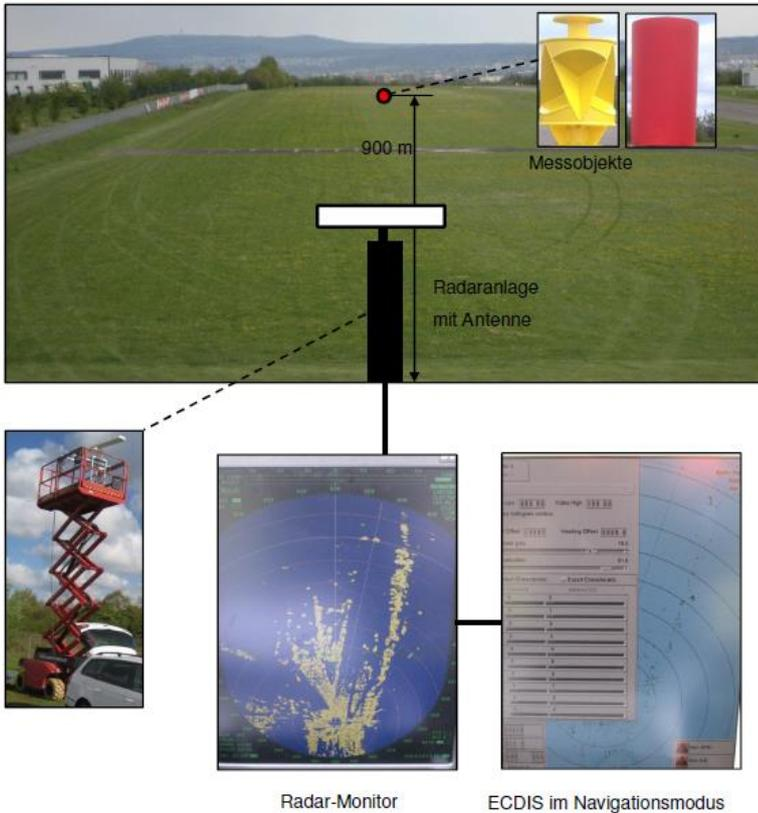
Figure 54 Setup for free field measurements on land
