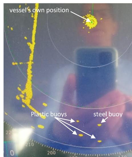
Figure 59 Radar picture, range ring distance 0.1 NM
