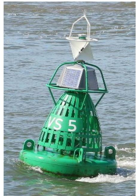
Figure 11 Steel buoy with radar reflector
