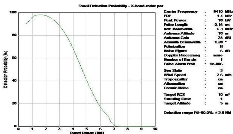
Figure 25 Detection probability with a typical non-SOLAS radar
