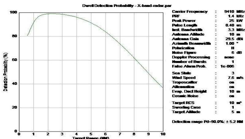
Figure 23 Detection probability with evaporation duct (height 10 m)
