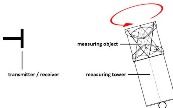
Figure 28 Radar reflector on measuring tower, elevation angle -10°
