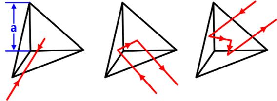
Figure 12 Reflection principle of a corner reflector
