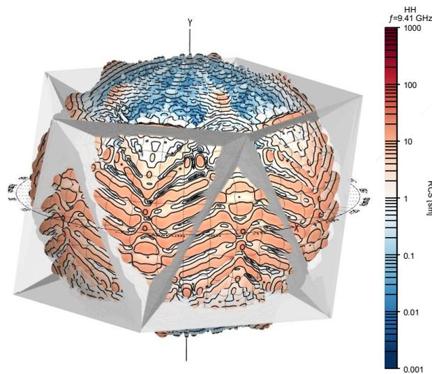
2D reflection diagram, different tilt angles, linear
