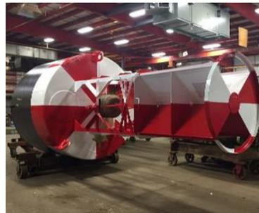
Figure 35 Radar reflector as part of the daymark
