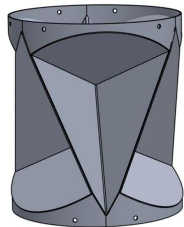
Figure 43 SR6 radar reflector
