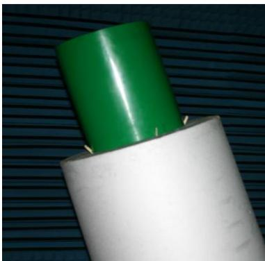
Figure 52 Radar reflector with plastic cover
