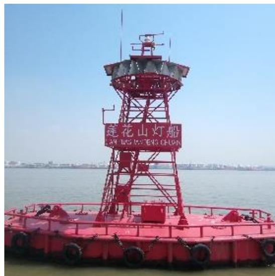
Figure 40 Corner reflectors on a LANBY
