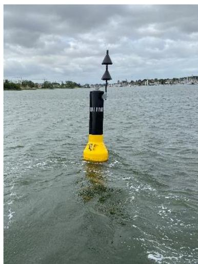
Figure 18 Plastic buoy with internal radar reflector
