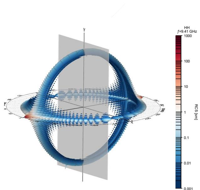
Figure 26 RCS simulation for a metal sheet
