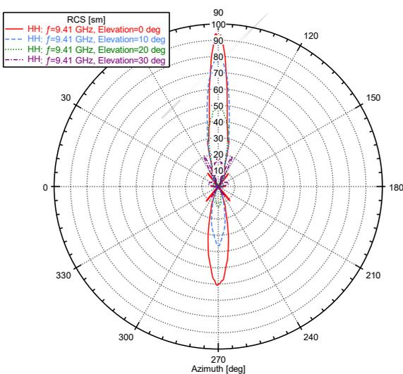
**2D reflection diagram, different tilt angles, logarithmic**
