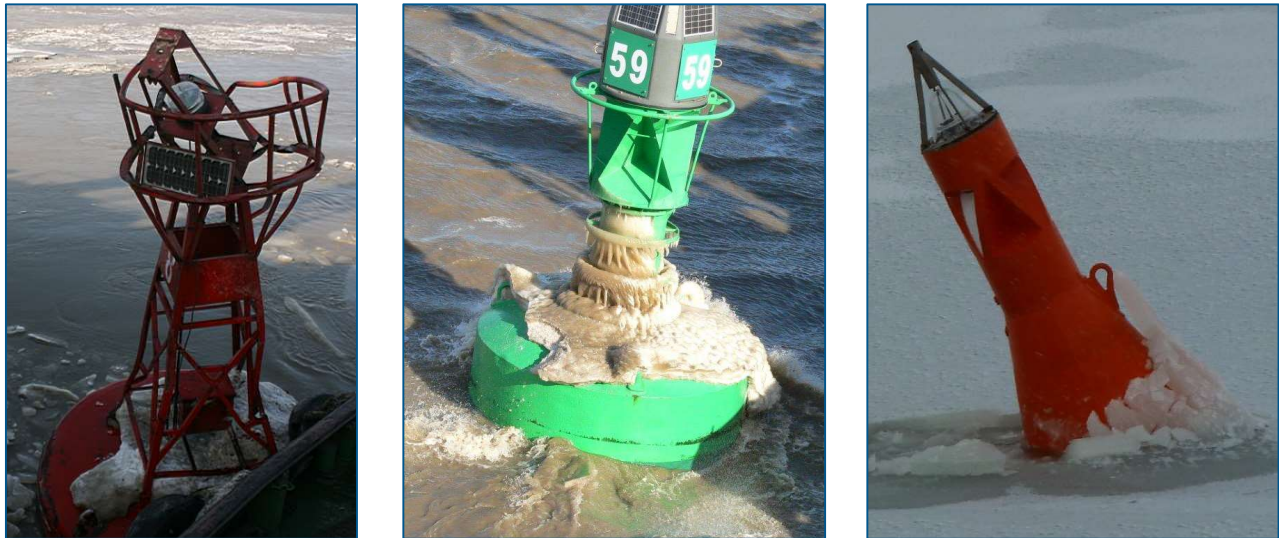
Figure 10 Effect of ice on buoys
