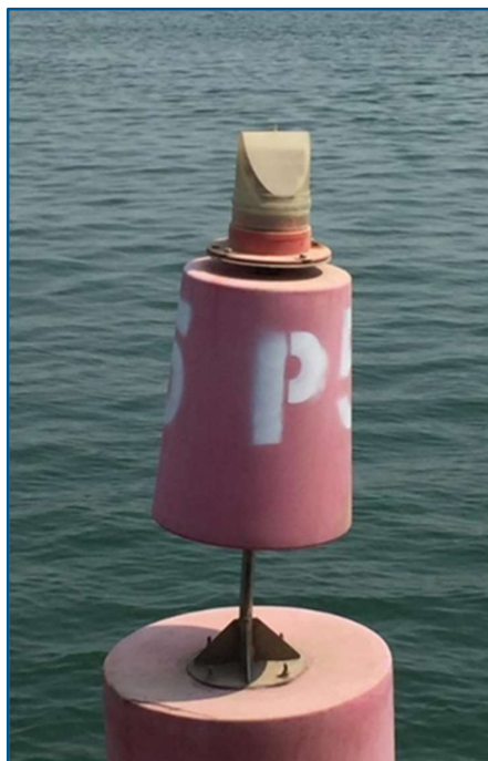
Figure 9 High Ultraviolet effect on red buoy
